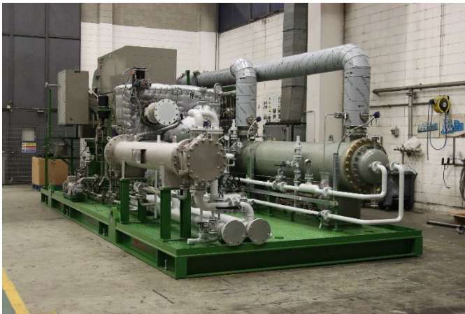
API 672 Centrifugal compressor
