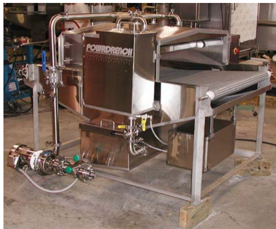
Figure 2. Surface application of liquid smoke by use of spray or drench system.
