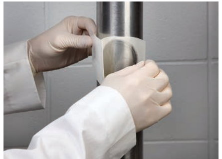
Figure 1. Examples of direct contact and swab sampling using 3M™ Petrifilm™ Plates
