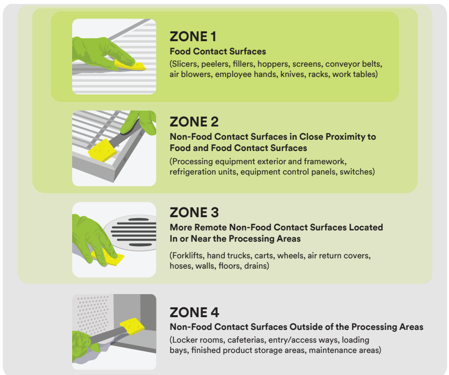
Figure 1. Environmental monitoring sampling zones
