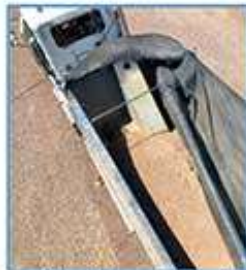
A truck driver fell 9 1/2 feet while adjusting the tarp. He had climbed up the side of the truck into the bed and fell while walking on loose sand.
