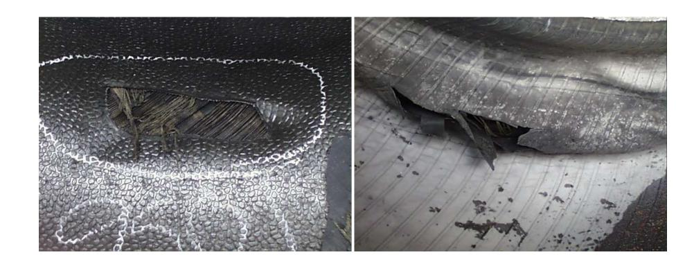
Do not inflate a tire that has been run flat without dismounting and inspecting it internally.
