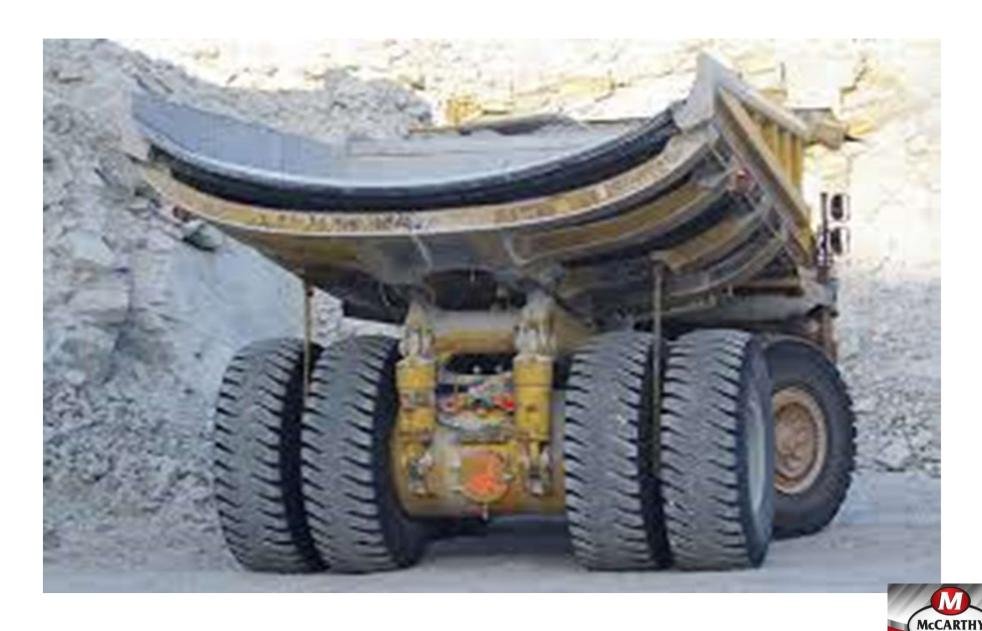
Prock ejectors wear over time and become very sharp. As they bounce off the sidewall of the tires, they will cut into sidewalls creating damage. Rock ejectors need to be inspected quarterly.
