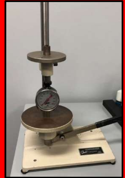
Durometer gauge used for testing hardness.
