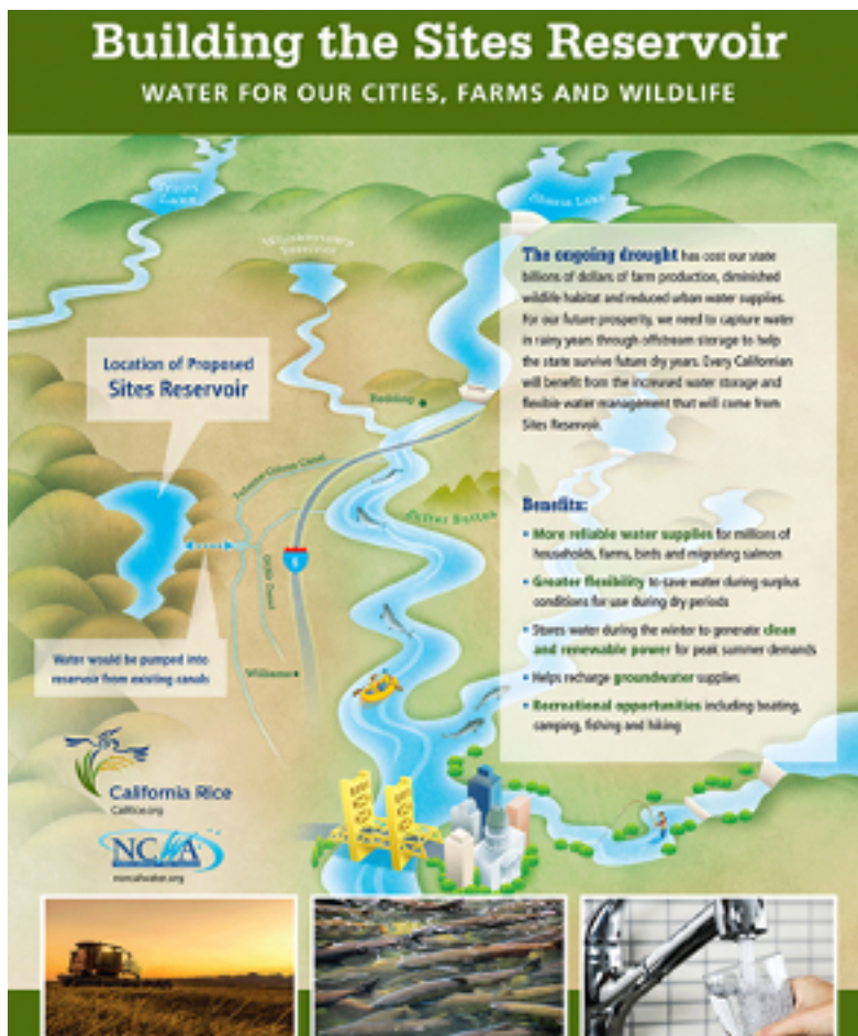
Figure 4. The new Sites reservoir would be an off-stream reservoir that would increase northern California's water storage capacity by up to 15 percent and help address the effects of climate change by increasing the flexibility, reliability, and resiliency of CVP and SWP.
