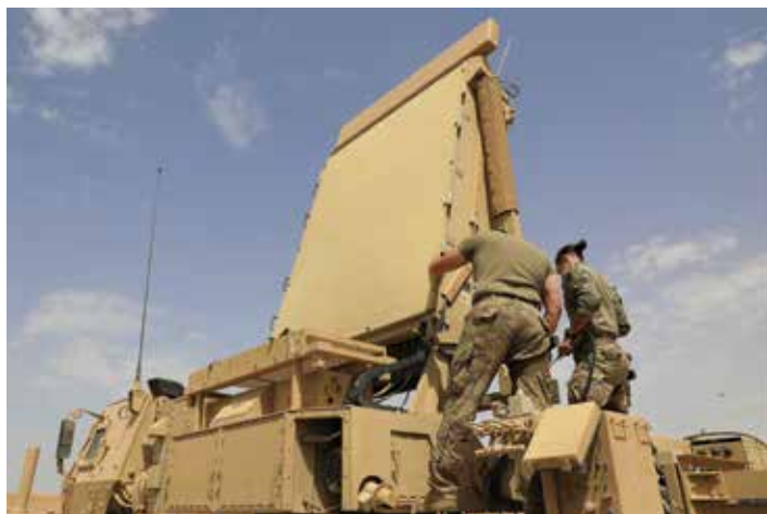
Members of the Target Acquisition Platoon, 130th Field Artillery Brigade, Task Force Spartan, conduct maintenance on the AN/TPQ-53 RADAR in the CENTCOM area of operation.
