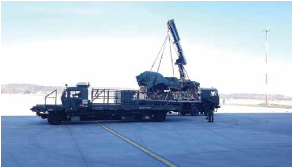
The truck transfers the Howitzers to a Polish Military K-Loader, which loads both platforms onto one C-130J.
