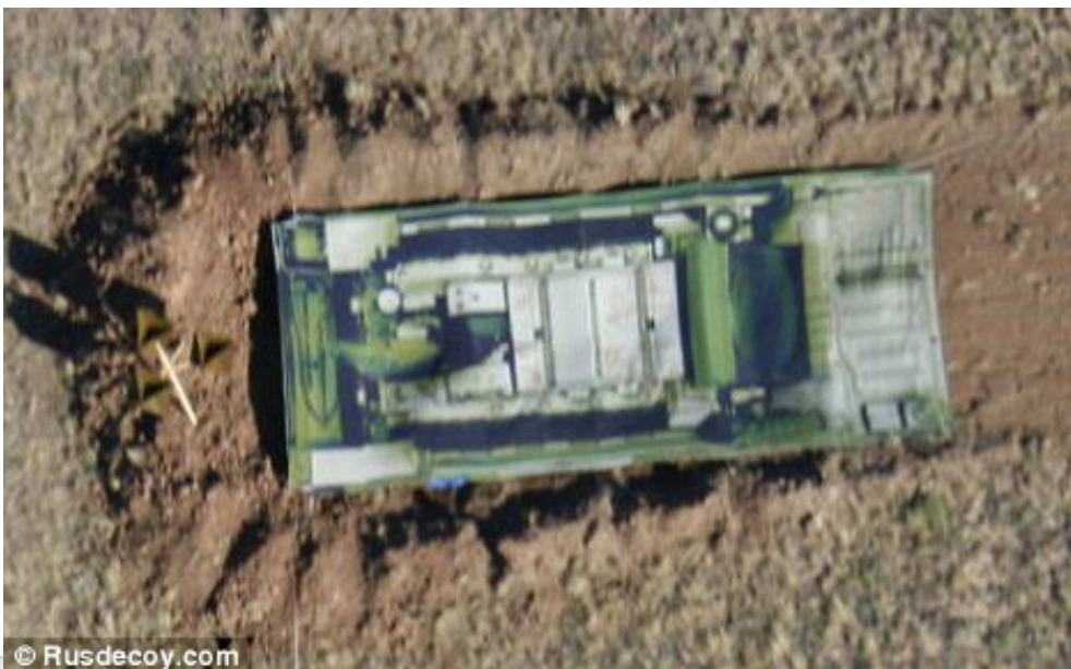
In conflicts of the future inflatable vehicles like the one above will be arrayed in defensive positions, under camouflage nets, and posted forward in critical points on the battlefield with the intent to disrupt the enemy's tempo. Source: Rusdecoy.com
