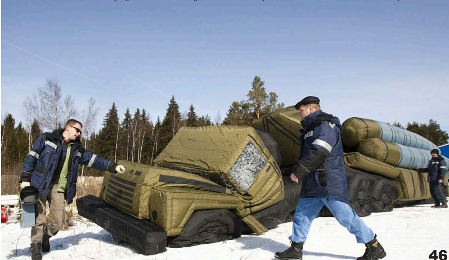
Workers inflate a model of a Russian S-300 long range surface-to-air missile system at the compound of the RusBal balloon manufacturer outside Moscow. The small firm produces infrared and radar reflective inflatable dummy targets in 1:1 ratio that are designed for the Russian military and the international defence market. Source: UK Daily Mail
