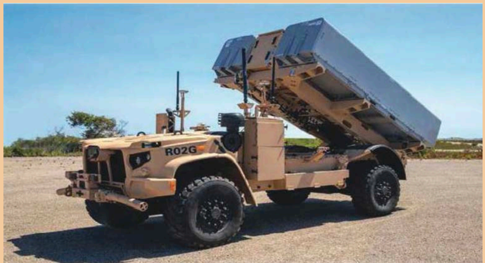
Ground Based Anti-Ship Missile (Naval Strike Missile) mounted on the Joint Light Tactical Vehicle. (Photo: Courtesy Marine Corps Systems Command.)
