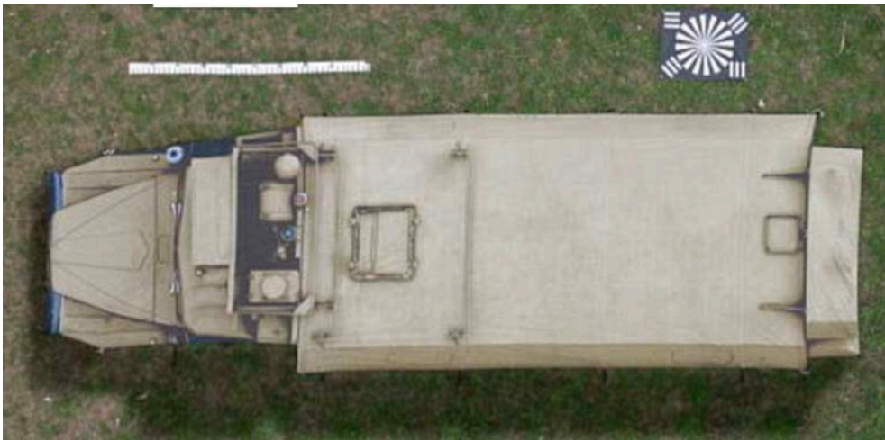
Another Russian firm, Rusbal, created this dummy of a truck, designed to look like the real thing from the air Source: Rusdecoy.com
