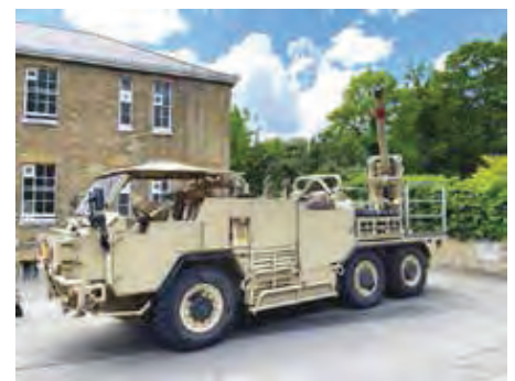
105mm L118 Light Gun, without muzzle brake, installed on a SUPACAT Extenda
