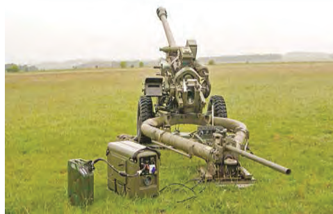
Royal Artillery 105mm L118 Light Gun Fitted with Leonardo Laser Inertial Artillery Pointing System.
