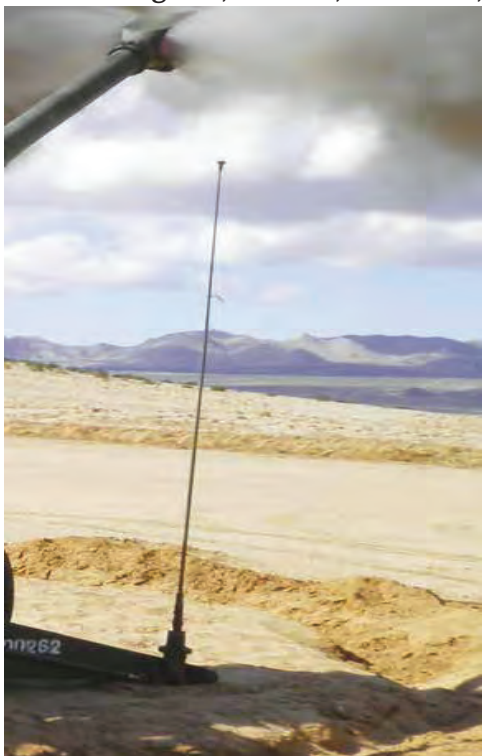
The M777 155mm/39 cal Light Towed Howitzer carrying out a fire mission and showing muzzle velocity radar mounted above ordnance.
