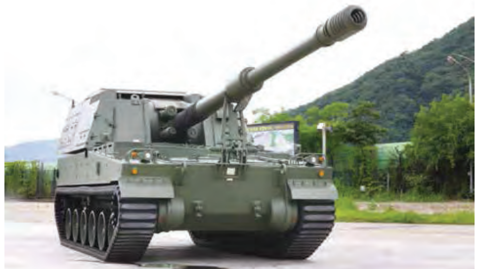
The South Korean Hanwha K9 Thunder is being adopted by an increasing number of countries and has undergone continuous development. This is the K9A2 with a Soucy Composite Rubber Track.
