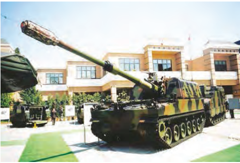
The Turkish Army deploys the locally manufactured Firtina 155mm/52 cal SP artillery system which is based on the South Korean Hanwha K9 and shown here with its Poyraz Ammunition Resupply Vehicle to the rear
