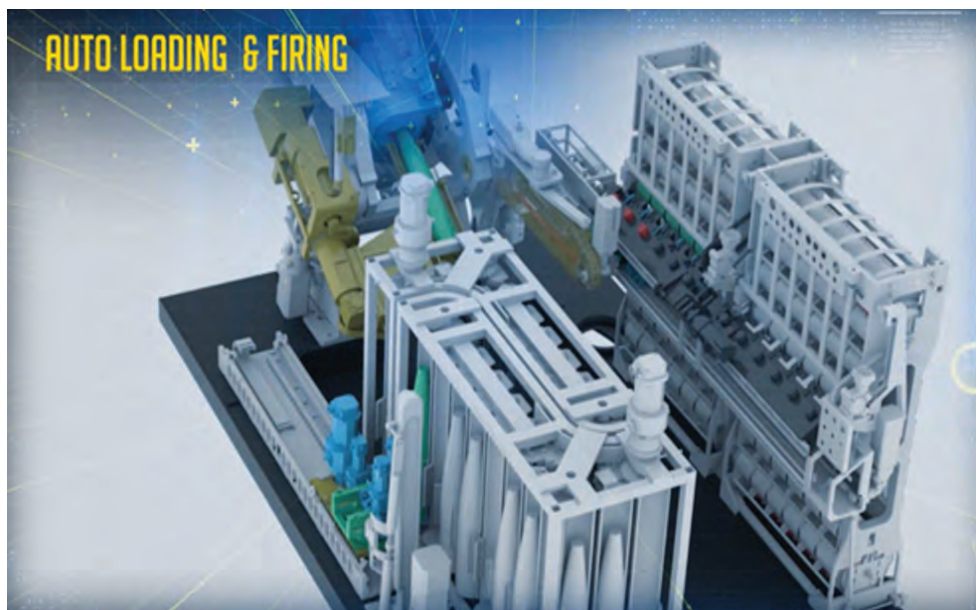
The Sigma Autoloader features dual projectile carousels and two independent charge magazines for redundant ammunition management.
