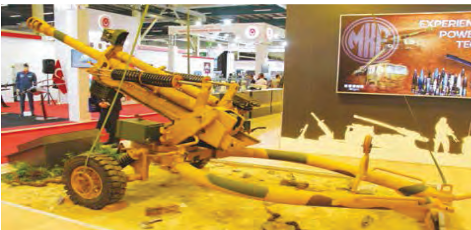
The latest 105mm towed artillery system to enter production is the 105mm Boran Air Transportable Light Towed Howitzer developed to meet the requirements of Turkey.
