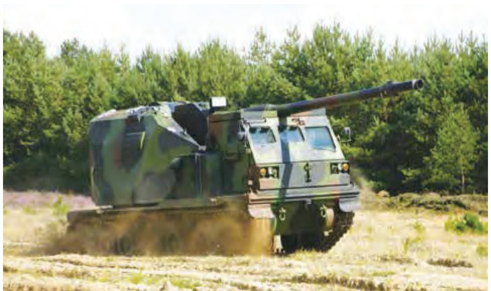
155mm/52 cal Artillery Gun Module installed on a M270 MLRS carrier chassis for trials
