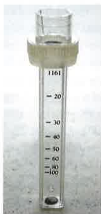
Photo 8-5. Calibrated cell for turbidimetric testing.
