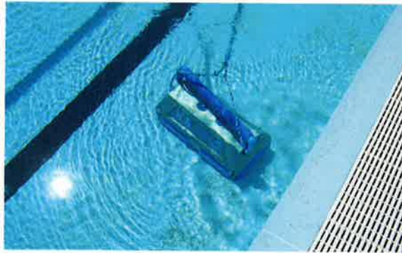
Photo 16-5. Larger pools may benefit from the use of an automated vacuum system.
