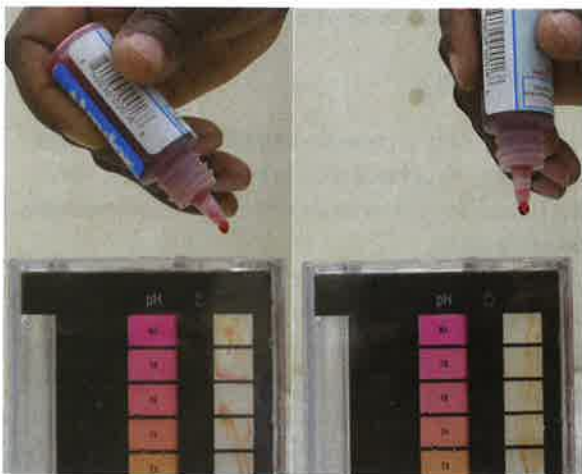
Photo 8-9. Reagent bottles should always be held in a vertical position to ensure the correct drop size.
