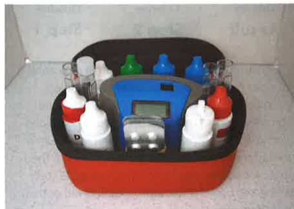
Photo 8-14. Photometric testing is ideal for use by pool operators who have problems discerning slight color differences.
