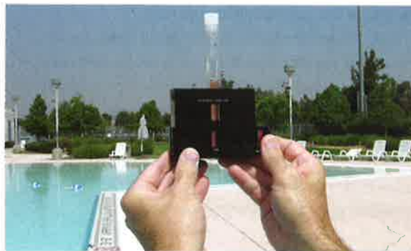
Photo 8-10. The comparator test block should be held up at eye level to the horizon opposite the sun for the best comparison to the printed standard.
