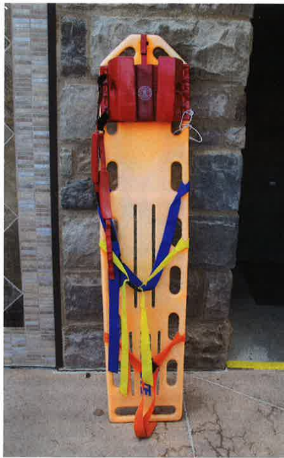
Photo 14-14. Most codes require a facility to have a backboard to respond to spinal injuries.
