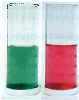
Photo 8-17. The normal beginning (green) and end (red) point for the titration of total alkalinity.
