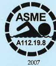
Illustration 14-1. Example of markings that must be visible on a drain cover.
