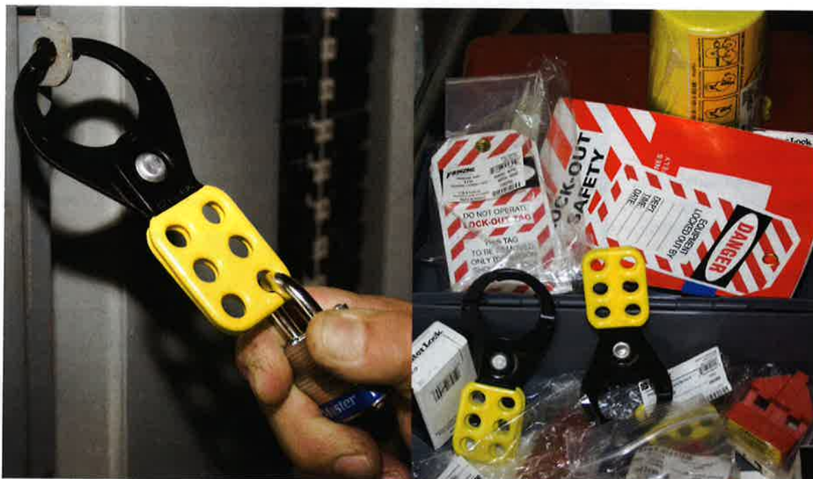
Photo 14-27. LOTO is the physical restraint or limit of all hazardous energy sources that supply power to a piece of equipment, machinery, or system.
