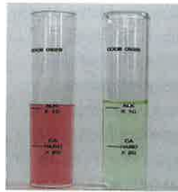
Photo 8-18. The normal end point (red) and false end point (yellow) for the titration of total alkalinity.
