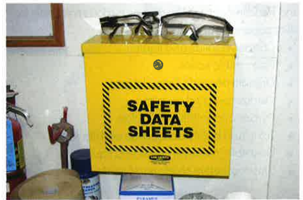
Photo 14-23. Use SDSs for guidance concerning the appropriate personal protective equipment.
