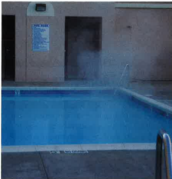
Photo 12-1. Evaporation is increased by high water temperature relative to the air temperature.
