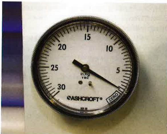
Photo 10-6. Vacuum gauges measure in inches of mercury or kilopascals.
