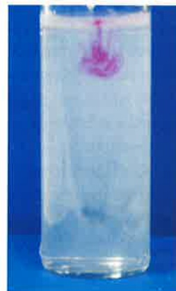
Photo 8-12. False DPD reading; if a temporary pink color appears, the sample water has a high chlorine content.
