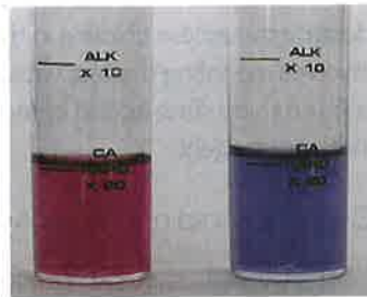
Photo 8-19. False calcium hardness endpoint
