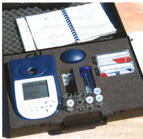
Photo 8-3. The photometer uses a beam of fixed wavelength light that is passed through the sample and the emerging light is analyzed electronically.
