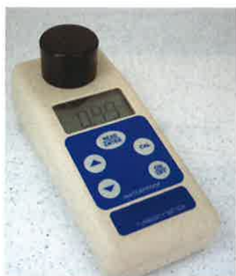
Photo 8-6. Handheld NTU electronic test meter
