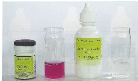
Photo 8-13. Titration DPD can easily determine chlorine concentrations as low as 0.2 ppm (mg/L) or as high as 20 ppm (mg/L).
