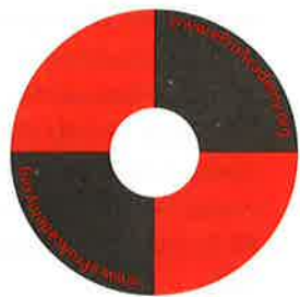
Illustration 8-1. Water clarity disk used to determine water turbidity
