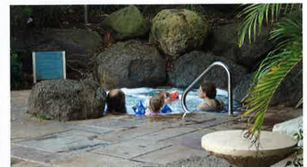
Photo 14-30. Spa user loads are usually based on one user for each 10 square feet (0.93 meters squared) of surface area.
