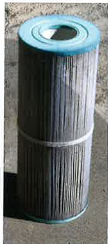
Photo 11-5. Cartridge filters elements are not backwashed, but cleaned.
