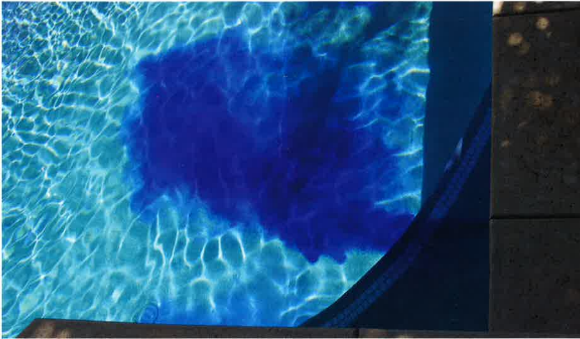
Photo 10-16. The design characteristics of some pools may require a dye test to insure proper water distribution patterns in every area of the pool.
