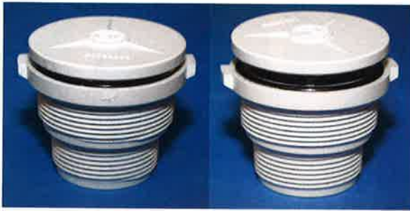
Photo 16-8. When ground water begins to exert pressure on the pool shell, the valve opens and allows the water to flow into the pool.
