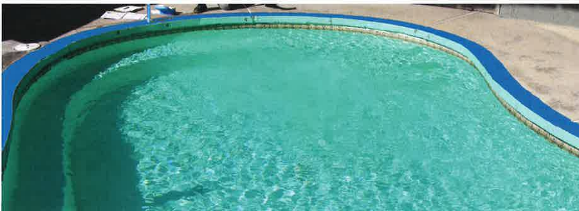
Photo 3-2. The volume of a kidney-shaped pool is calculated using the area x average depth x 7.5.
