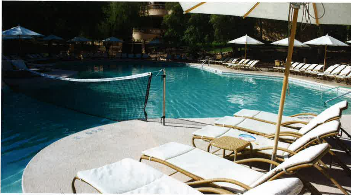
Photo 15-6. The opening checklist will assure that proper clearance is maintained around the pool. Most states regulations require a clearance of 4 feet.
