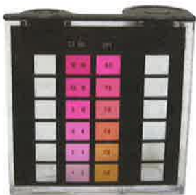
Photo 8-1. The most common form of testing uses a colorimetric test block with printed standards.
