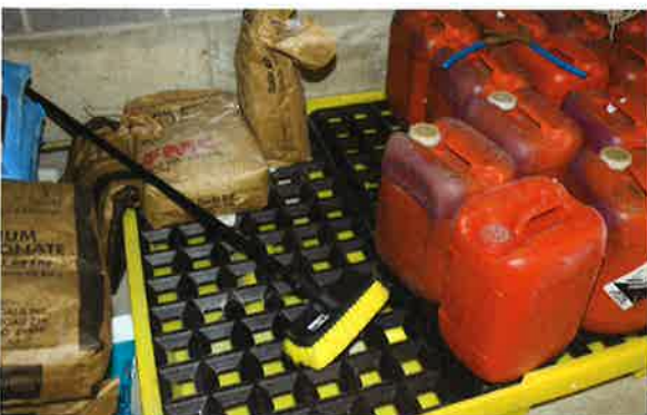
Photo 2-1. Improper storage of chemicals could result in dangerous chemical reactions.
