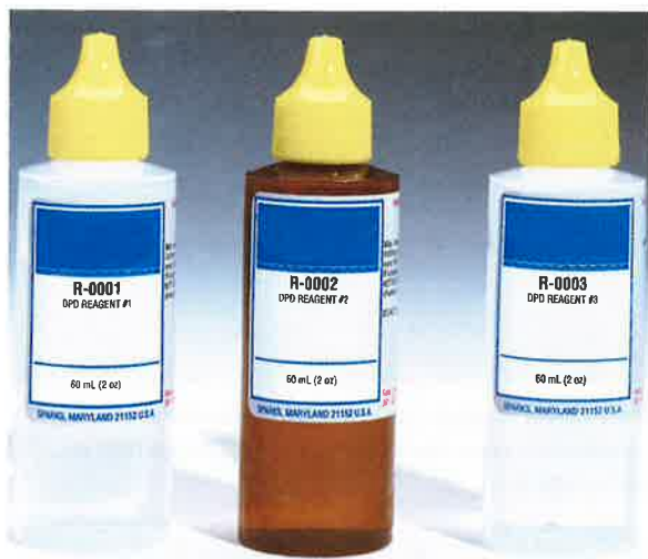
Photo 8-11. DPD has the capability of measuring both free and total chlorine.
