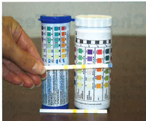
Photo 8-4. Dip-and-read test strips have a comparison standard printed on the packaging.
