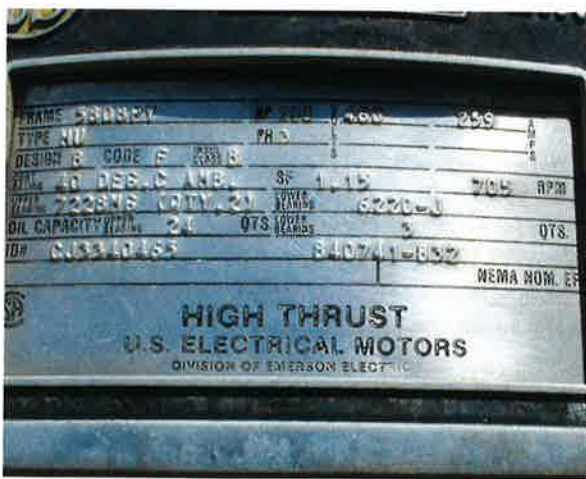
Photo 15-7. Digital photographs of motor data plates maybe useful to record in case the motor needs to be replaced.
