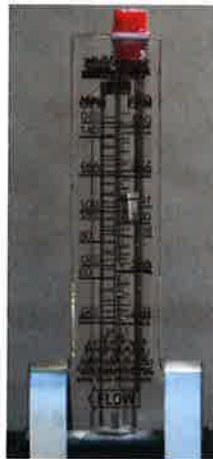
Photo C1-3: Flow meters must be installed correctly and calibrated regularly.
