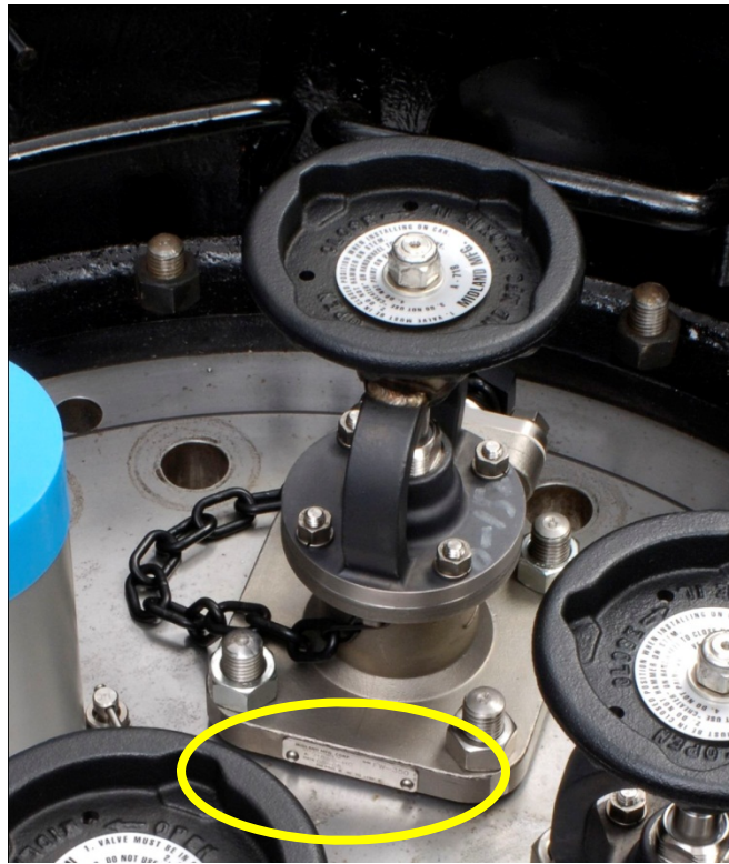
Figure 3: Location of Nameplate on Midland Dual Valves
