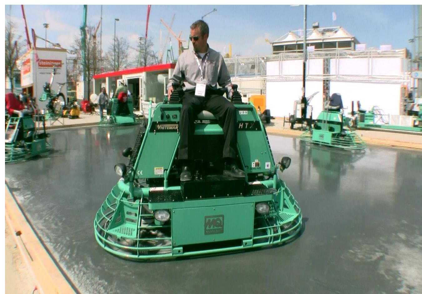
Ride-on trowels are used in the same way as walk-behind machines but allow for much larger areas to be floated and troweled by a single operator. They also minimize surface imperfections like footprints and generally provide smoother, flatter floors than walk-behind machines. See Pages 66-70 for important information on machine floating and troweling.
