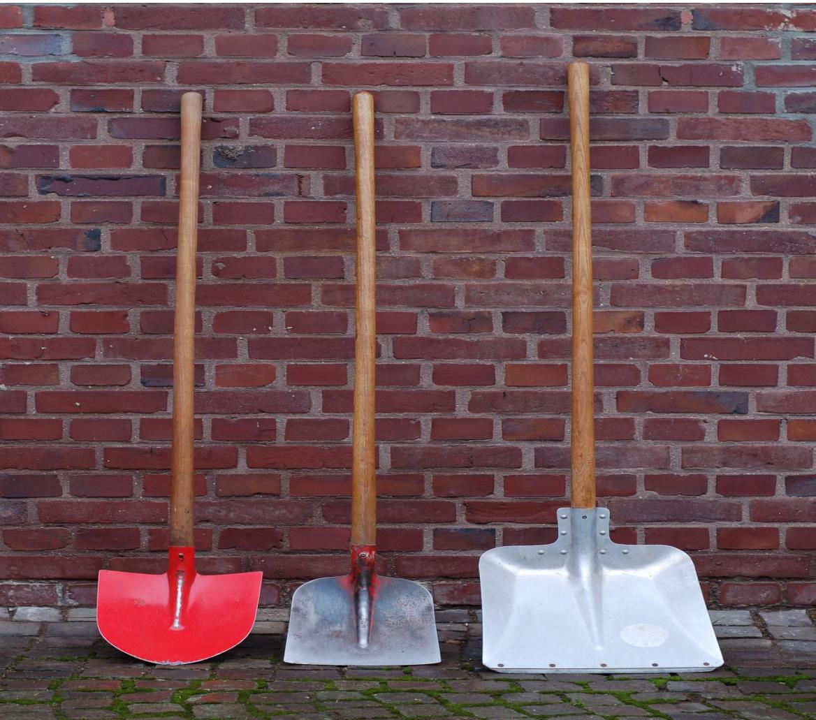
Only the center shovel (above) is an appropriate tool for use with fresh concrete. The square shovel can move concrete with minimal segregation and can also be used for rough leveling of concrete in smaller areas.
