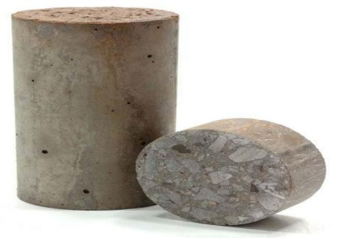
Most test cylinders today are made using molds that are 4" in diameter and 8" tall. Once made, the cylinders should be covered with a plastic cap and placed in an area away from vibration, movement and extreme temperatures.
