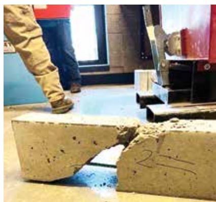
Break Result of FRP Beam Design
