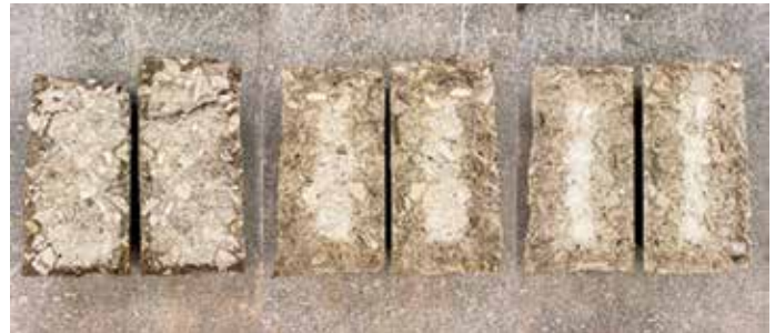
Figure A-4: Deicing Salt Penetration After 280 Days in 4" x 8" Cylinders (a) Commercial 3500 Both (b) Commercial Both (c) CRED Both
