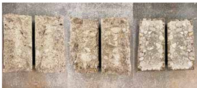
Figure A-3: Deicing Salt Penetration After 280 Days in 4" x 8" Cylinders (a) Commercial 3500 +2Gal/CY (b) Commercial ACI +2Gal/CY (c) CRED +2Gal/CY
