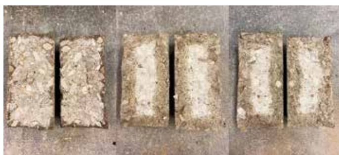
Figure 2: Deicing Salt Penetration After 280 Days in 4" x 8" Cylinders (a) Commercial 3500 No Cure (b) Commercial ACI No Cure (c) CRED No Cure
