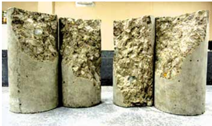
Figure 1: Pumice Compressive Strength Cylinders (25% substitution right and 35% substitution left)
