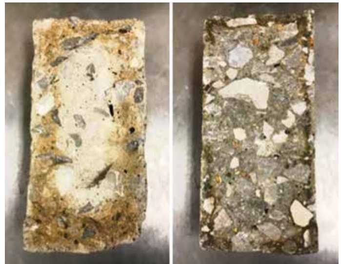
Figure 2: Magnesium Chloride Salt Solution Penetration Depth in 4-by-8-inch Cylinders (a) 3500-psi (b) CRED Level 1
