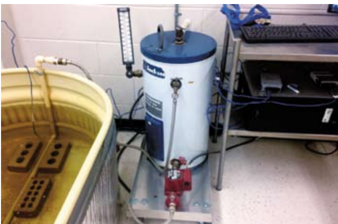
Figure 6: Close Up of Water Heater for Accelerated Curing Tank
