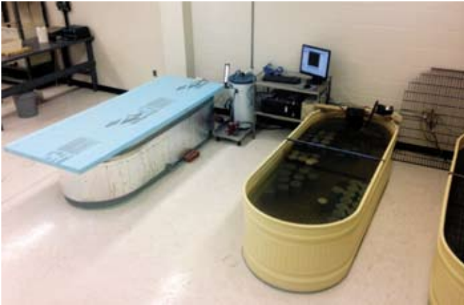
Figure 4: Accelerated (left) and Normal (right) Curing Tanks for the Project
