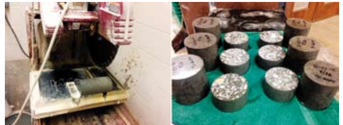
Figure 5: Water-cooled Saw and Sawed Specimens for RCP
