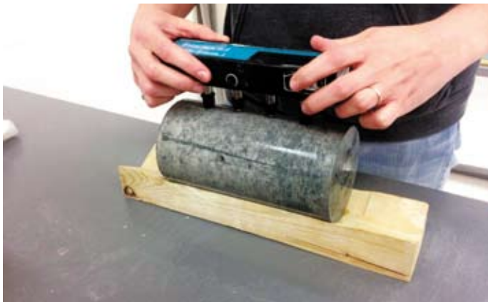
Figure 3: Conducting Surface Resistivity on Required Non-conductive Cradle
