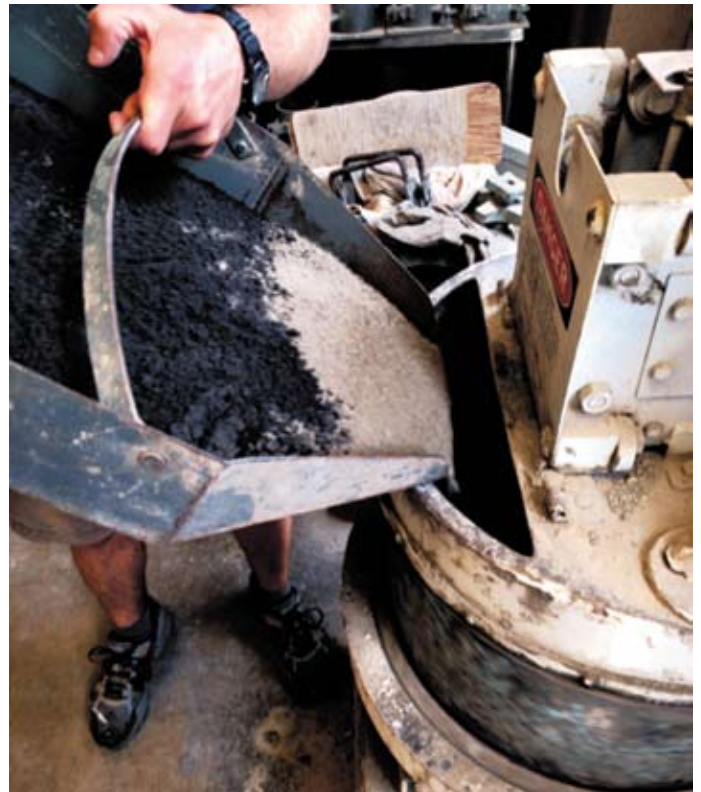
Figure 2: Loading PC and Bad Ash into the Mixer
