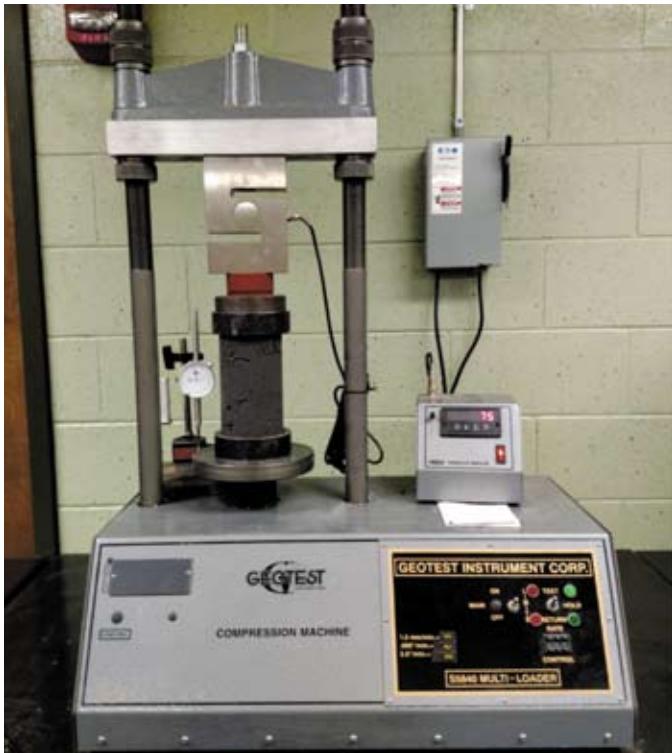
Figure 4: Compression Testing of Bad Ash Flowable Fill
