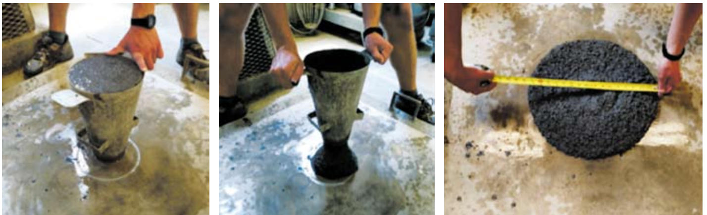
Figure 3: Inverted Slump Flow Testing of Bad Ash Flowable Fill
