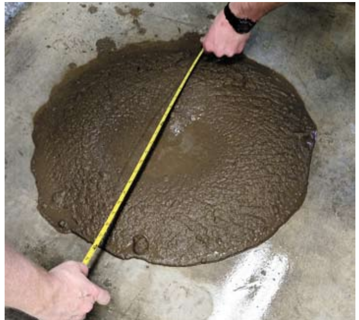
Figure 3: Patty Formed by Proper Flowable Fill Diffusion
