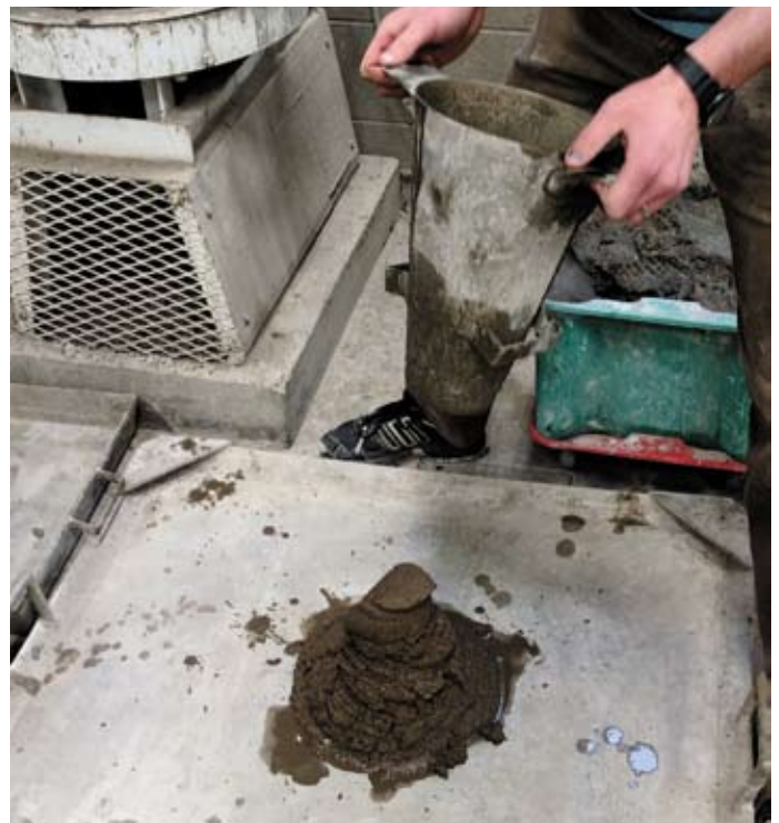
Figure 4: A "Did Not Flow" Result for an Inverted Slump Cone Consistency Test
