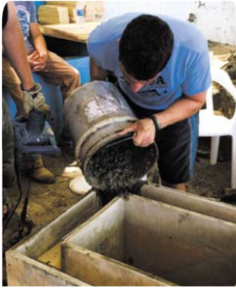
CIM junior, Nick Langlois, pours concrete into a prism form.
