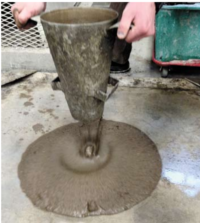
Figure 2: Raising the Inverted Slump Cone
