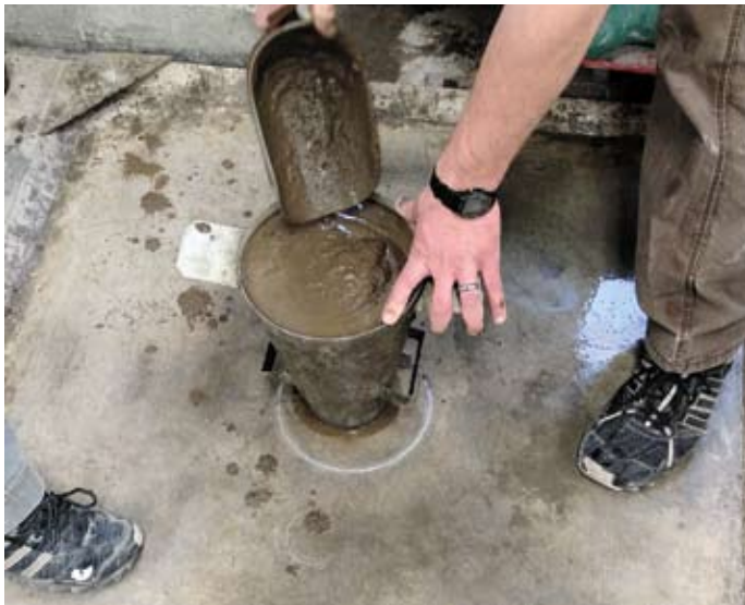
Figure 1: Filling the Inverted Slump Cone
