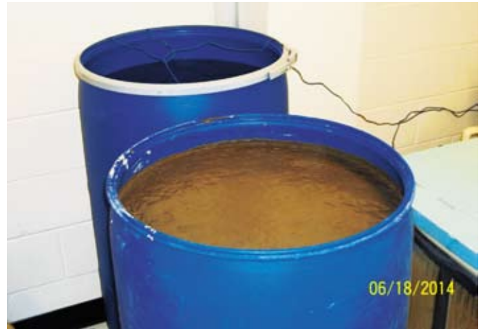
Figure 9: Less Expensive "Field" Test for Heat of Hydration Comparison
