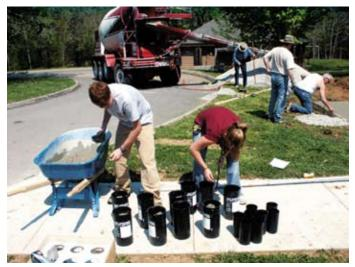
Figure 4: Making Test Cylinders, Finishing and Cleaning Up
