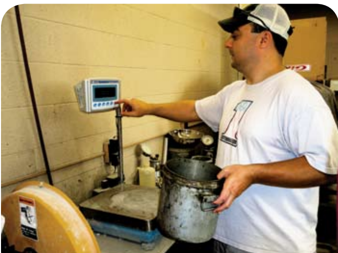
Figure 3: Determining Mass of Measure for ASTM C 1688
