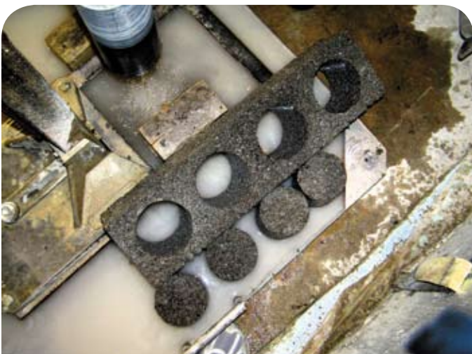
Figure 8: Cored Pervious Concrete Beam and Four Cores
