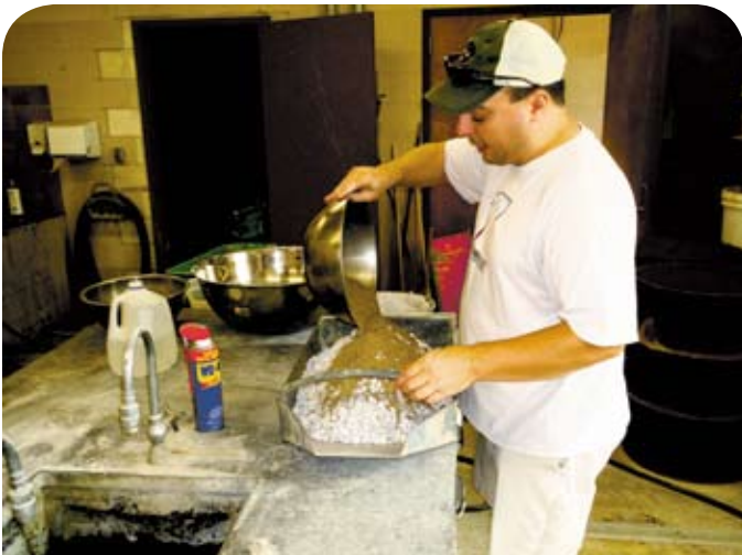
Figure 2: Preparing a Small Laboratory Batch for ASTM C 1688
