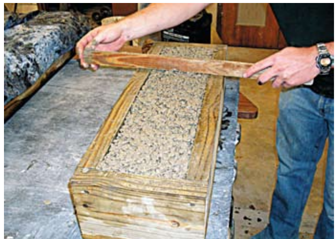
FIGURE 3: STRIKING OFF SELF-COMPACTING PERVIOUS BEAMS IN THE LABORATORY
