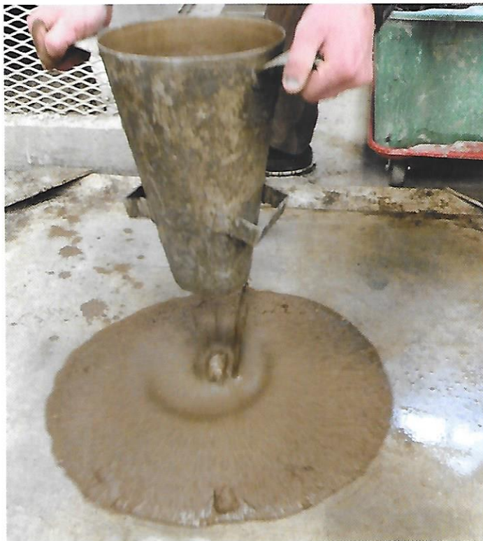
Figure 2: Raising the Inverted Slump Cone
