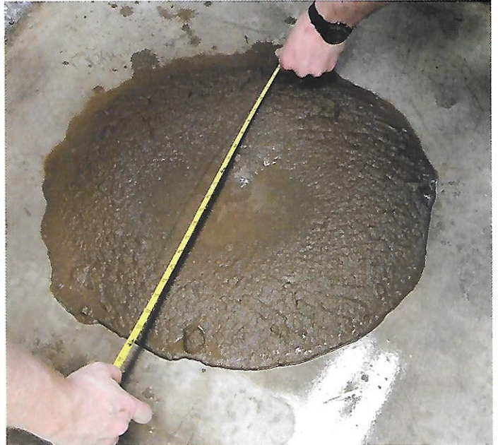
Figure 3: Patty Formed by Proper Flowable Fill Diffusion
