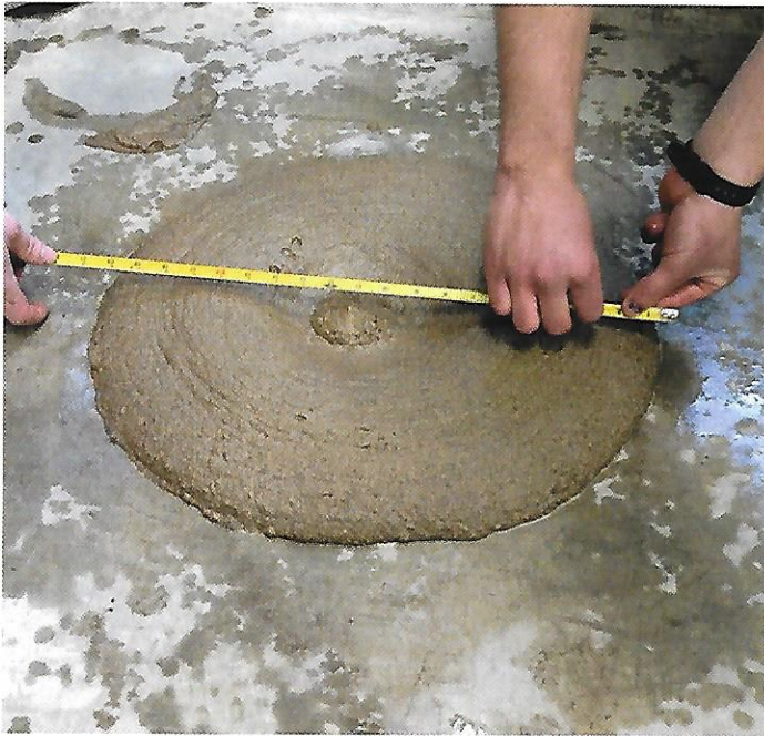
Figure 5: Inverted Slump Cone Consistency Test of an Air Entrained Mixture
