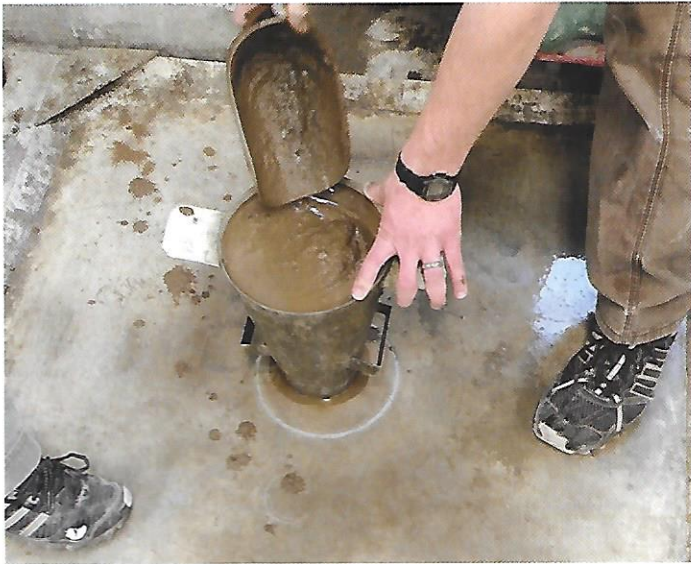
Figure 1: Filling the Inverted Slump Cone
