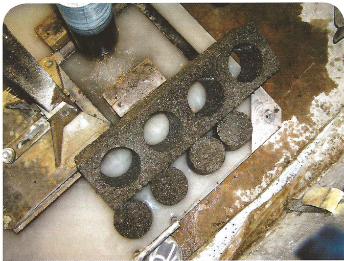
Figure 8: Cored Pervious Concrete Beam and Four Cores
