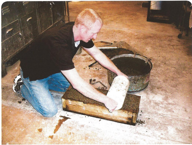
Figure 7: Compacting a Beam with a 6x12-inch Concrete Cylinder Roller
