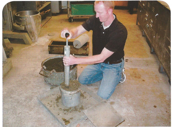
Figure 4: Preparing a Small Laboratory Batch for ASTM C 1688
