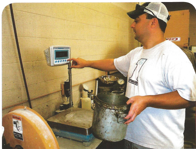
Figure 3: Determining Mass of Measure for ASTM C 1688
