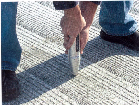
A rebound hammer can indicate relative concrete strengths but cannot directly measure compressive strength in the field.
