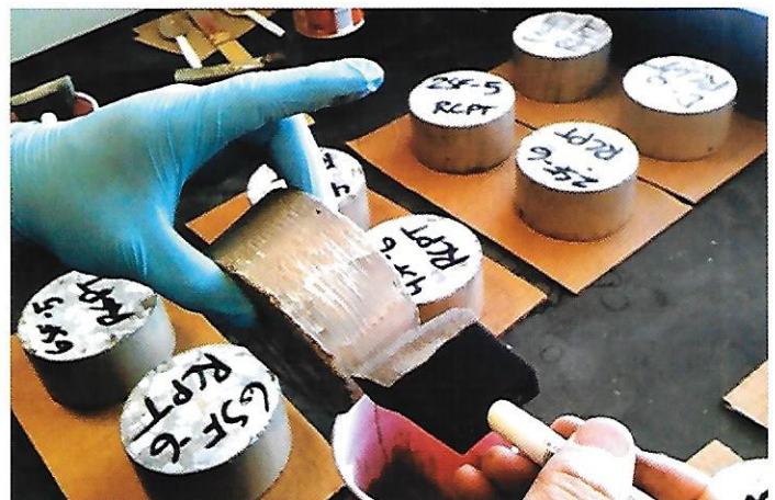
Figure 6: Epoxy Coating of 2-inch Slices for RCP Test
