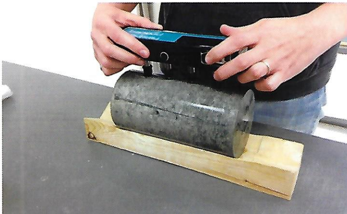
Figure 3: Conducting Surface Resistivity on Required Non-conductive Cradle
