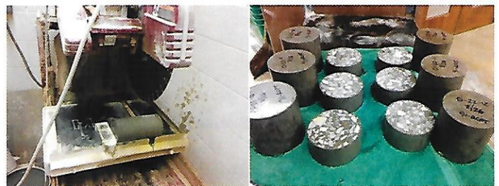
Figure 5: Water-cooled Saw and Sawed Specimens for RCP
