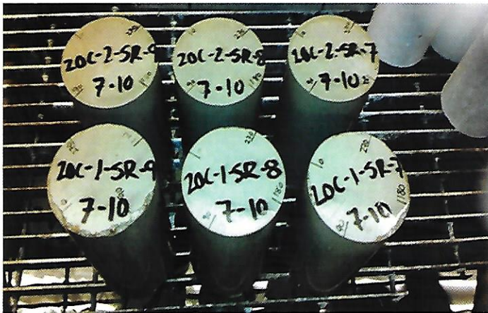
Figure 2: 4x8-inch Cylinders Marked for Conducting Surface Resistivity Testing
