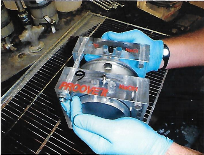
Figure 7: Chemical Reservoirs in RCP Test Cells
