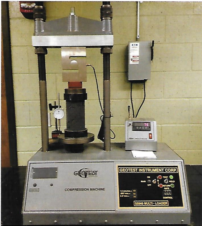
Figure 4: Compression Testing of Bad Ash Flowable Fill
