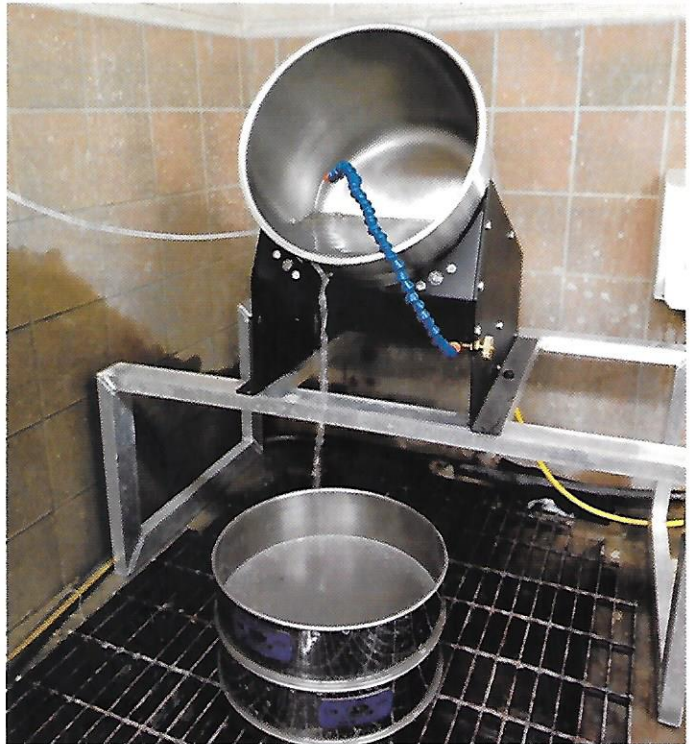
Figure 1: Washing Screenings for Sieve Analysis
