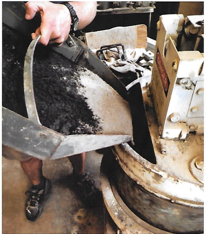
Figure 2: Loading PC and Bad Ash into the Mixer
