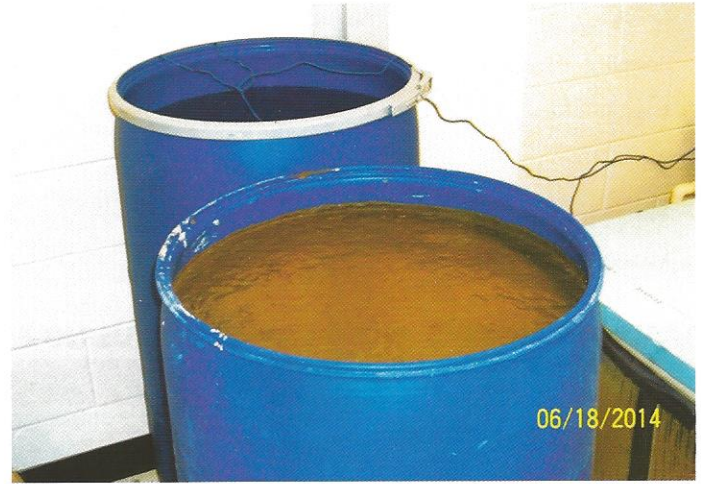
Figure 9: Less Expensive "Field" Test for Heat of Hydration Comparison
