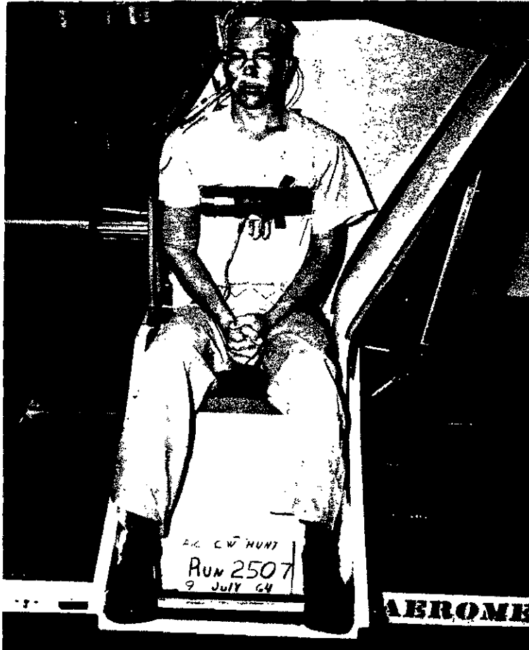
FIGURE 3. Instrumented subject in Seat Prior to Test.
