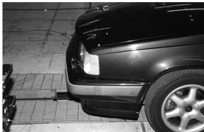
Figure 4 - Bumper Surface Damage after the 11.21 kph Impact.
