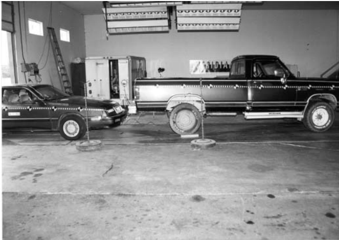
Figure 10- The LeBaron to pickup Impact Configuration.
