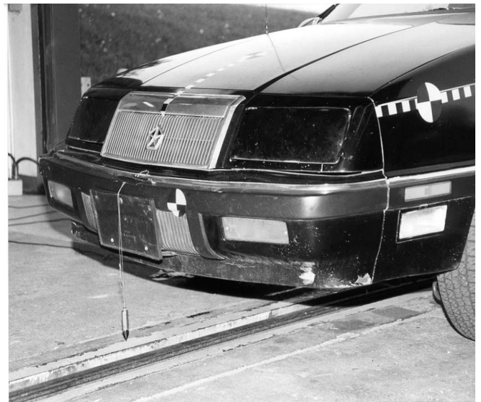
Figure 12 - Undamaged LeBaron. Target shows Hitch Ball Impact Point.
