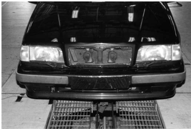
Figure 4 - Bumper Surface Damage after the 11.21 kph Impact.
