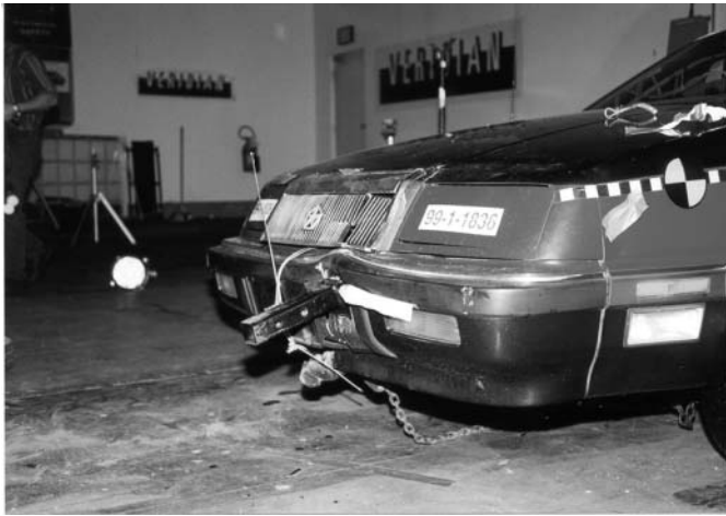
Figure 17 - External Damage in the 17.74 kph Impact
