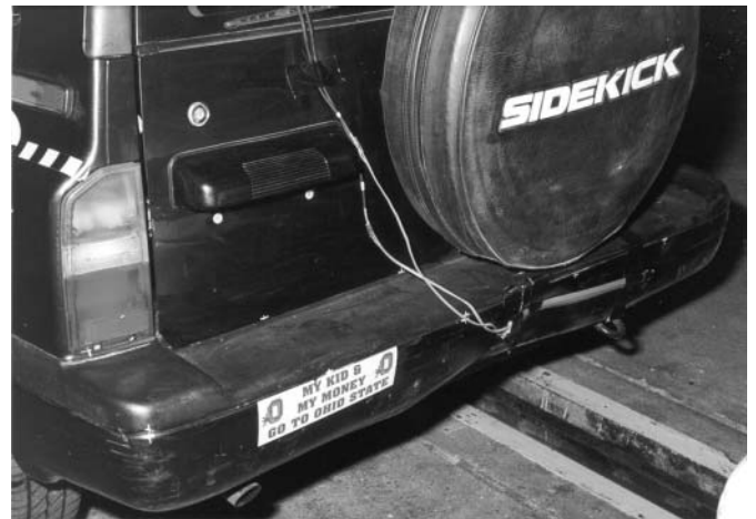
Figure 32 - Suzuki Damage in the 17.91 kph Impact
