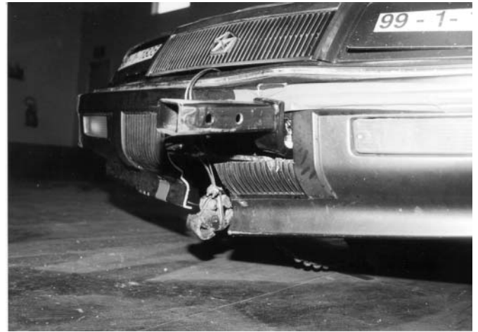
Figure 15 - External Damage in the 11.45 kph Impact.
