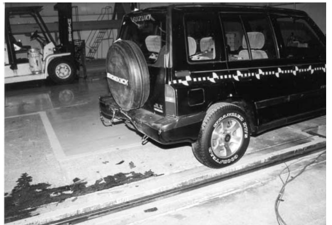
Figure 33 - Suzuki Damage in the 32.42 kph Impact
