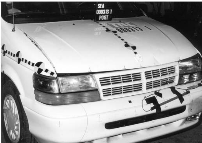
Figure 30 - Grand Caravan Damage in the 17.91 kph Impact
