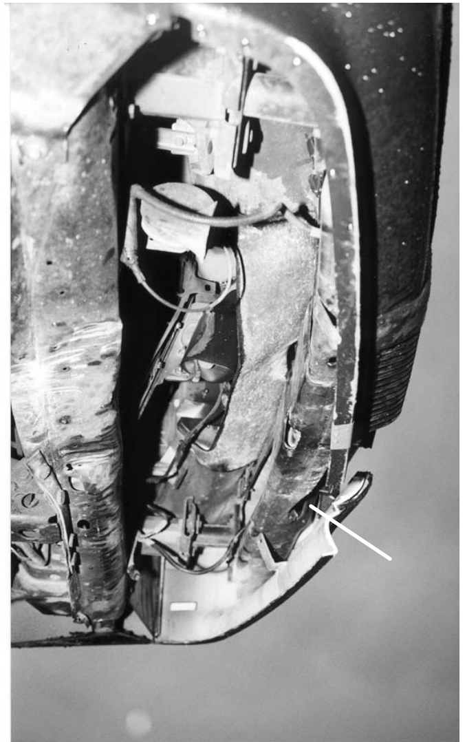
Figure 16 - Reinforcement Bar Damage from the 11.45 kph Impact
