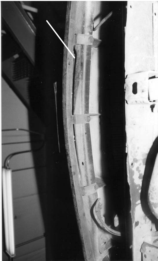
Figure 14 - Reinforcement Bar Damage from the 11.29 kph Impact
