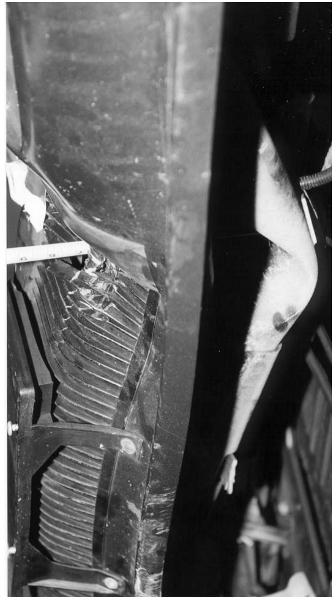
Figure 20 - Reinforcement Bar Damage in the 19.35 kph Impact.
