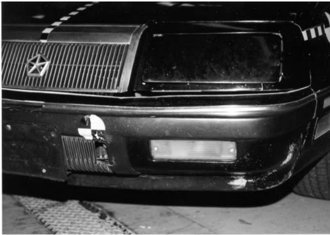
Figure 13 - External Damage in the 11.29 kph Impact. Target indicates Hitch Ball Impact Position.
