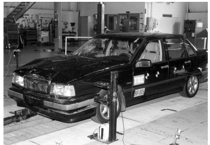
Figure 7-Side View of the 20.89 kph Impact Damage.
