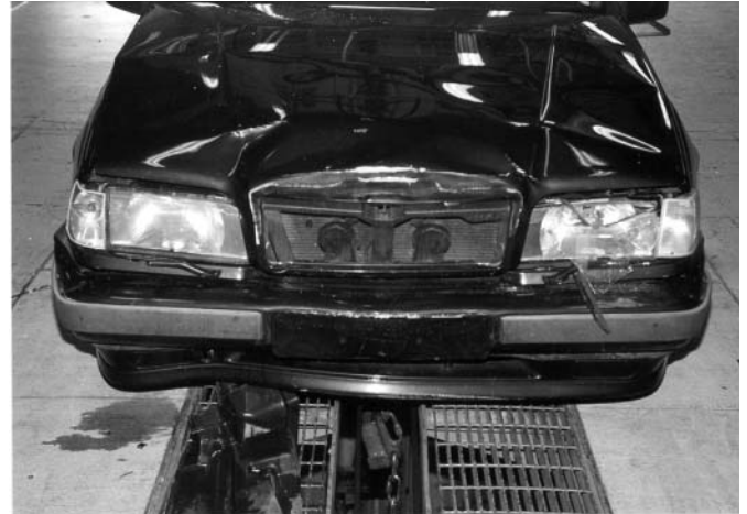
Figure 6-Damage After the 20.89 kph Impact.
