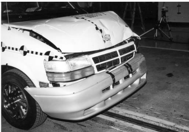
Figure 31 - Grand Caravan Damage in the 32.42 kph Impact
