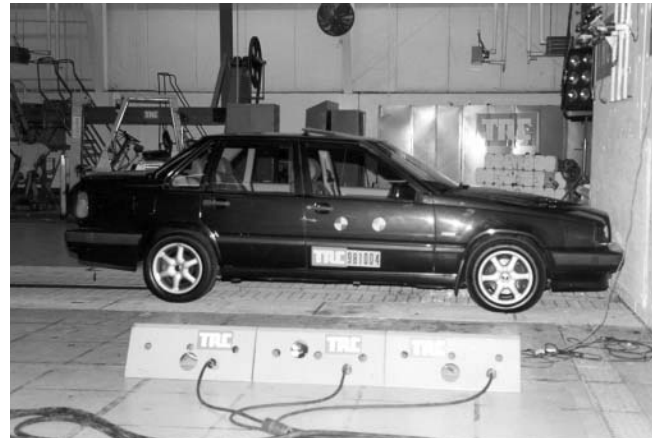
Figure 1 - 1993 Volvo 850/Barrier Impact Configuration
