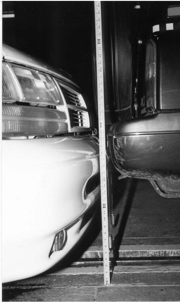
Figure 23 - Impact Configuration of the Grand Caravan into the Suzuki Sidekick.
