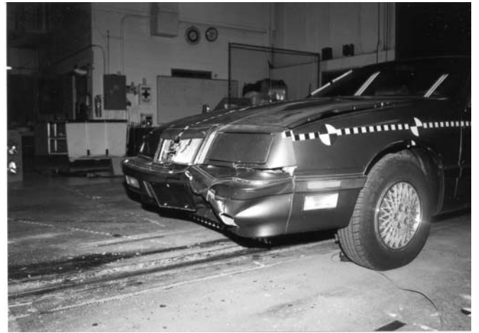
Figure 19 - External Damage in the 19.35 kph Impact
