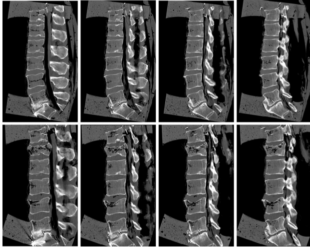
Fig. 6 Sagittal CT of the specimen subjected to higher severity acceleration pulses demonstrating burst fracture at L1 and anterior wedge fracture at L4. Top row images were obtained prior to dynamic testing and bottom row images were obtained immediately following the last test. The two images in each column were obtained from approximately the same medial-lateral position.
