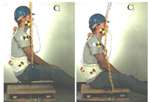
Figure 4. Video captures of a volunteer completing the seated drop activity from 100 mm.
