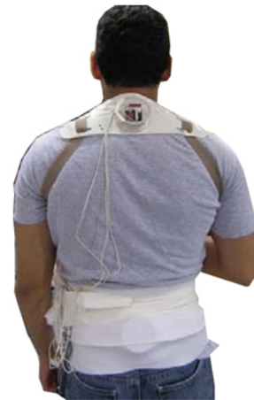
Figure 1. Tri-axial accelerometers attached to custom-fit mounts were securely strapped around the lumbar and upper thoracic regions.
