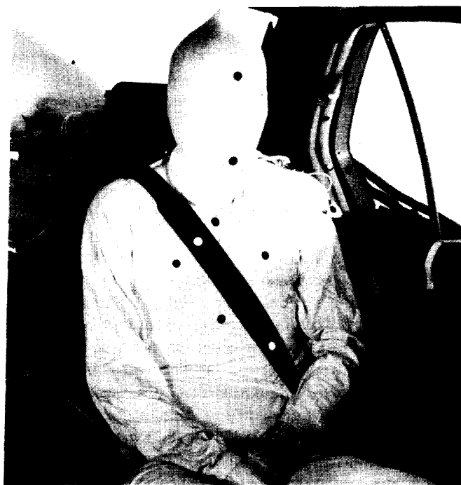
Fig. 2: Location of the optical targets at the body of the subject by the side collision tests
