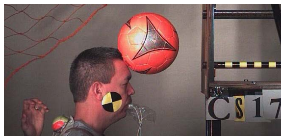
Fig. 2. Video capture of a soccer ball impact.
