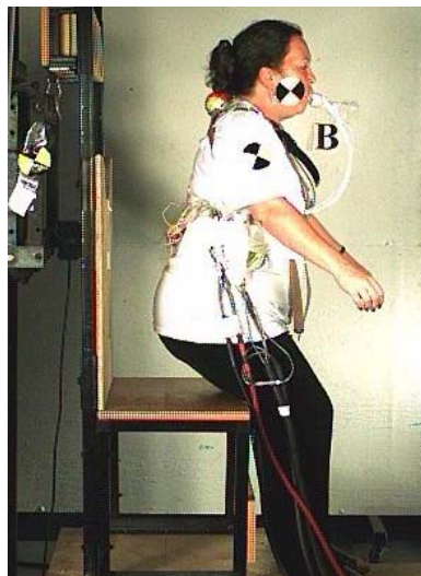
Fig. 5. Video capture of a seat plop.
