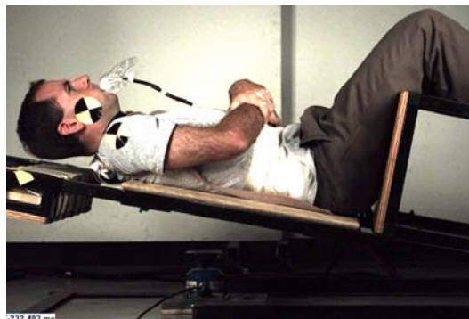
Fig. 6. Video capture of a chair tip from a height of 15 cm.
