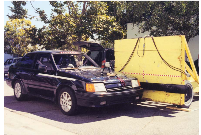
Figure 1 - Barrier/vehicle exemplar orientation
