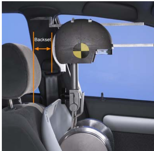
Figure 9 Measuring Backset for BioRID Set-up
