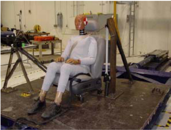
Figure A-1. Test set-up for the Lincoln rear impact tests. A Hybrid-III ATD was seated in the driver's seat mounted rigidly to the pneumatic sled used in the tests previously described. Tests delivered approximately 7.3 and 9.3 m/s (17 and 21 mph) delta Vs.
