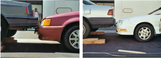
Figure 1: Exemplar pre-test override/underride configurations
