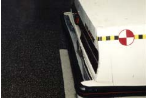
Photo 19. 3.8 m/s. Rear of Celebrity. Right side of bumper permanently crushed inward approximately one inch.
