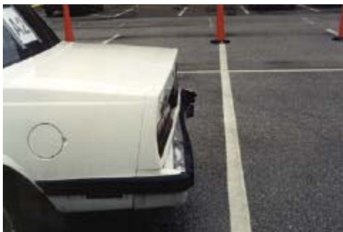
Photo 21. 4.2 m/s. Rear of Celebrity. Right side of bumper permanently crushed inward approximately three inches.
