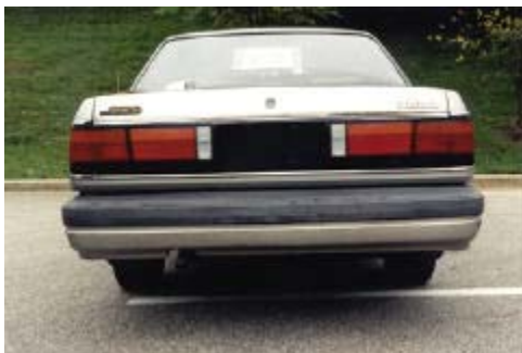
Photo 9. 4.6 m/s. Rear of Mazda. Bumper cover detached at right rear wheel well and bumper rotated downward slightly.
