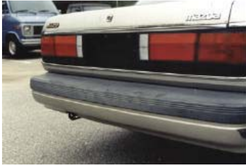
Photo 1. 0.8 m/s. Rear of Mazda. Minor blemishes to plastic bumper cover from Honda license plate mounting bolts. No permanent crush damage.
