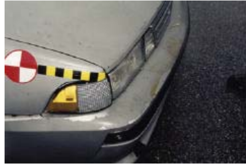
Photo 20. 3.8 m/s. Front of Cavalier. No permanent crush damage.
