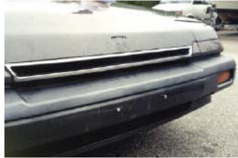
Photo 8. 4.1 m/s. Front of Honda. More pronounced scuffing. No permanent crush damage.
