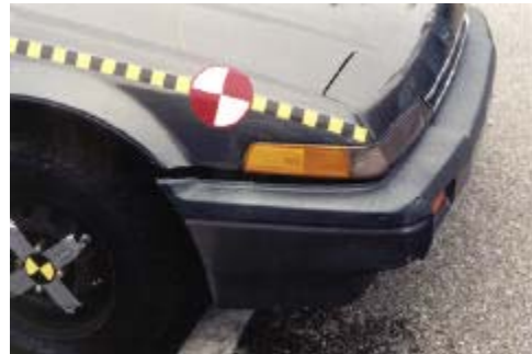
Photo 4. 1.6 m/s. Front of Honda. No permanent crush damage.
