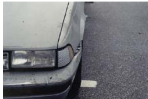
Photo 24. 5.8 m/s. Front of Cavalier. Additional permanent crush damage.
