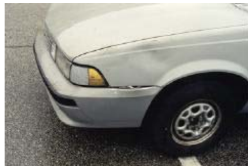
Photo 22. 4.2 m/s. Front of Cavalier. Some permanent crush damage.
