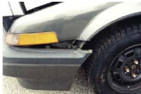
Photo 10. 4.6 m/s. Front of Honda. Permanent crush damage to left front corner of bumper.
