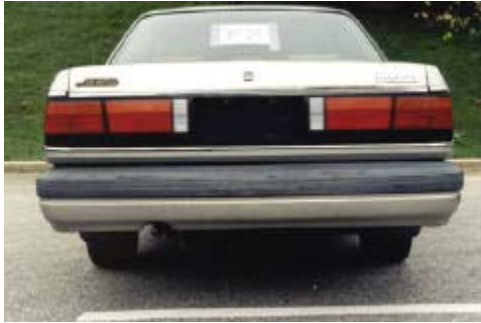
Photo 7. 4.1 m/s. Rear of Mazda. More pronounced scuffing. No permanent crush damage.
