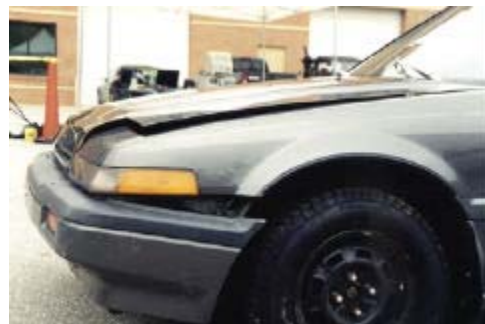
Photo 12. 5.0 m/s. Front of Honda. More severe damage, including buckling of engine compartment hood.
