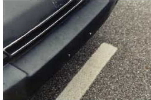
Photo 2. 0.8 m/s. Front of Honda. Note license plate mounting bolts. No permanent crush damage.
