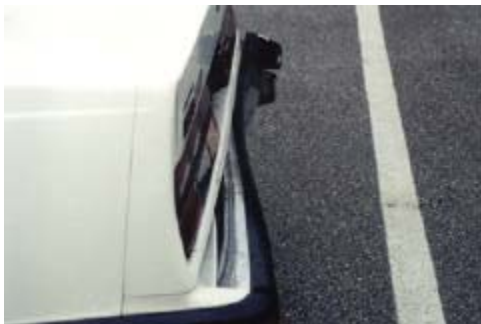
Photo 23. 5.8 m/s. Rear of Celebrity. Additional permanent crush damage.
