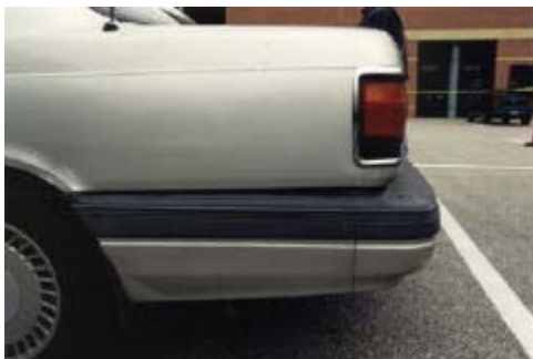
Photo 11. 5.0 m/s. Rear of Mazda. No additional damage noted.
