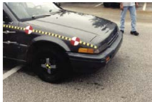
Photo 6. 2.9 m/s. Front of Honda. No permanent crush damage.
