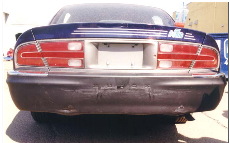
Photo D7 – Rear bumper cover of 1998 Buick Park Avenue exhibits more pronounced tow hook imprints and is flexed upward. Reinforcement beam and impact absorber displaced forward.
