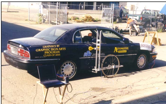
Figure 1 – Sintra Engineering 5 th Wheel Mounted to Buick Park Avenue for Vehicle-Vehicle Test
