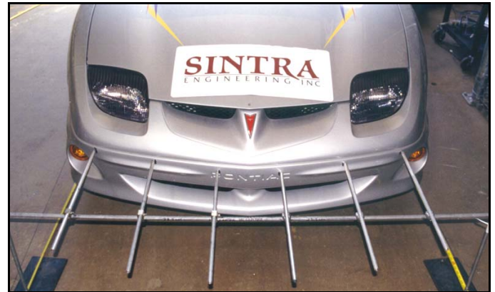
Figure 2 - Measurement Jig Aligned with Pontiac Sunfire's Front Bumper
