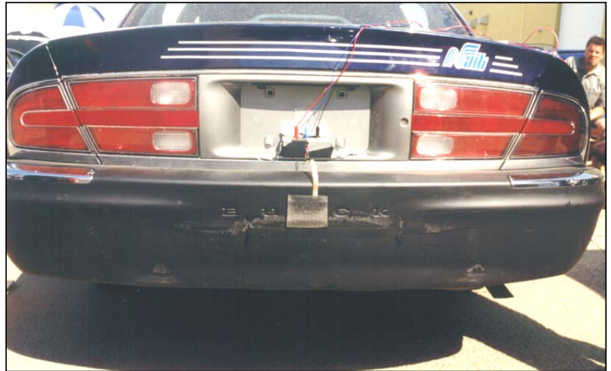
Photo D5 – Rear of 1998 Buick Park Avenue exhibits scuff marks and tow hook imprints on bumper cover.
