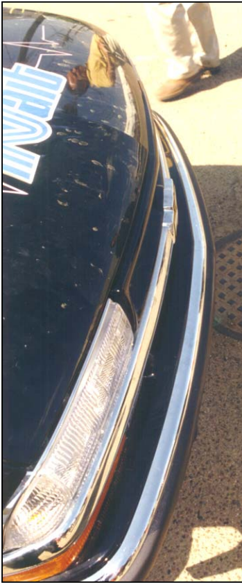
Photo D4 – Front face bar of 1999 Chevrolet Blazer displaced rearward by 6 mm.
