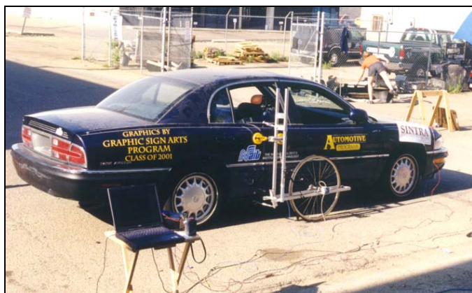
Figure 1 – Sintra Engineering 5 th Wheel Mounted to Buick Park Avenue for Vehicle-Vehicle Test
