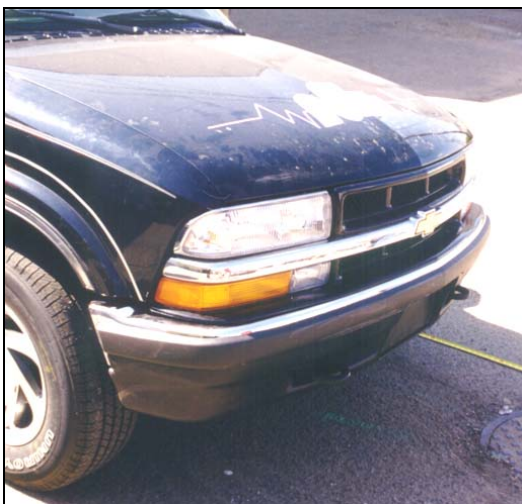
Photo D6 – Front face bar of 1999 Chevrolet Blazer tilted downward and displaced rearward by 12 mm. Lower portion of face bar is also locally deformed.
