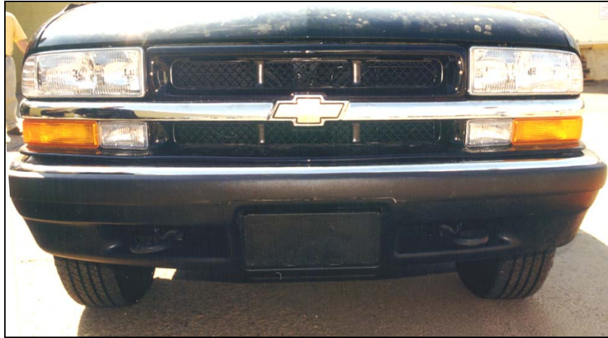
Photo D1 – Front of 1999 Chevrolet Blazer exhibits minor scuff marks on impact strip.
