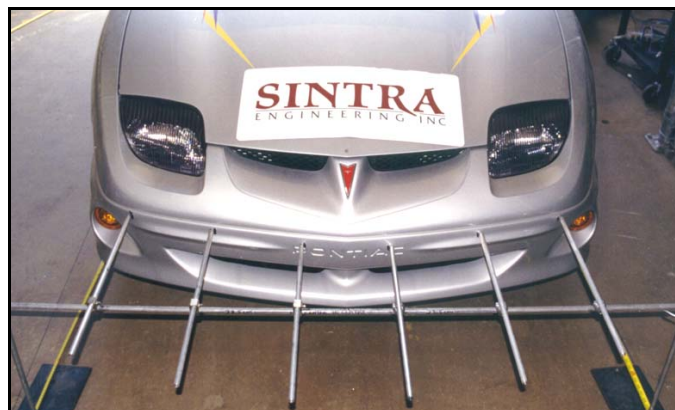
Figure 2 - Measurement Jig Aligned with Pontiac Sunfire's Front Bumper
