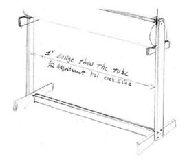
**Figure 4:** Support feet on each end of the base can be any length, but no less than 24." The feet will need to be longer the taller the rack is built.
