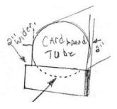
**Figure 3:** The rack base should be 1" longer than the tubes it will be holding. Allow for 1/2" on each side of tube
