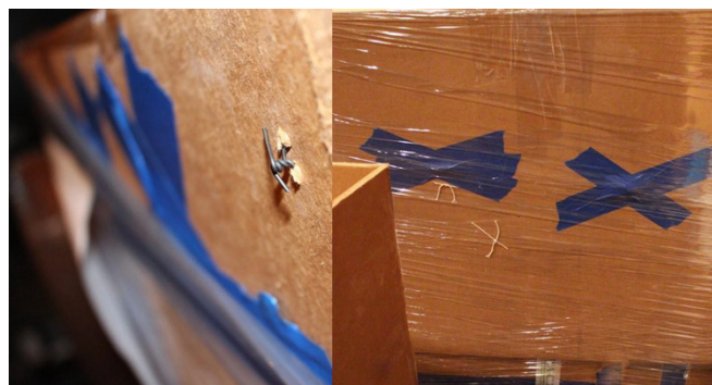
Figure 5: Twist the wires to secure the specimen to the box. Tape over the twisted wire to avoid any snags or cuts.
