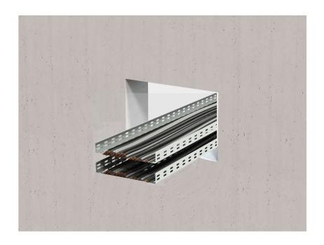
Cable Trays Through 2HR Fire-Rated Concrete Floor or Wall Assembly
