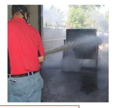
To pass test, must not produce any though-gaps in firestop system
